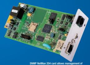
UPS across LAN using any of the main network communication protocols: TCP/IP; ModBus TCP/IP;
